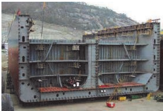
A section of a ship's hull showing the double bottom. This vessel also has double sides, so as well as tanks below the cargo area, saddle tanks sit beside it.
